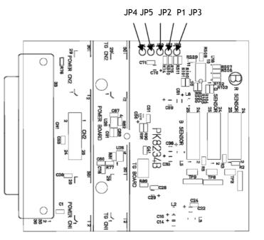
Fig. 21. Potentiometers and jumpers placing
